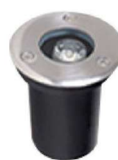
NO:YF-DMD-01 510 Outer diameter size: Φ65x80MM Inner diameter: Φ35MM Hole size: Φ60MM Power: 1W Shell material: die cast aluminum
