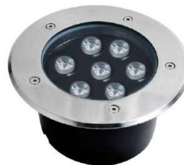
NO:YF-DMD-05 1335 Outer diameter size: Φ150x90MM Inner diameter: Φ85MM Hole size: Φ128MM Power: 7W Shell material: die cast aluminum
