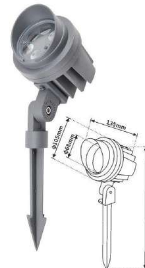
NO:YF-PZDC-12 12W 2530 Outer diameter size: Φ105MM Inner diameter: Φ68mm Power: 3W/6W Shell material: die cast aluminum
