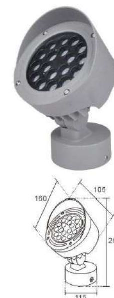
NO:YF-xHDZ-06 24W 3960 36W 4650 Shell material: die cast aluminum Product size: 160x105x255MM Aluminum substrate size: 120MM Power: 12/18x2W Power box size: 123x50xH40MM
