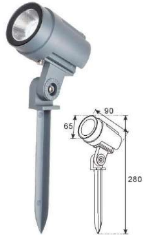
NO:YF-PZDC-01 5W 1565 7W 1610 10W 1725 Shell material: die cast aluminum Product size: 65x90xH280MM Aluminum substrate size: 47MM Power: COB 5W/7W/10W Power box size: 50x30xH45MM
