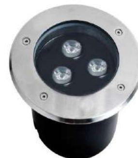
NO:YF-DMD-02 970 Outer diameter size: Φ80x80MM Inner diameter: Φ50MM Hole size: Φ75MM Power: 3W Shell material: die cast aluminum
