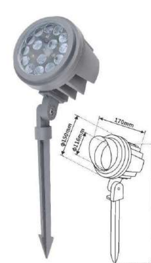
NO:YF-PZDC-13 30W 4255 Outer diameter size: Φ150MM Inner diameter: Φ116mm Power: 9W/12W/15W/18W Shell material: die cast aluminum
