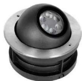
NO:YF-NYD-01 2255 2645 2415 Product size: 200x185x140MM Aluminum substrate size: 68MM Power: 3W/5W/6W Shell material: die cast aluminum
