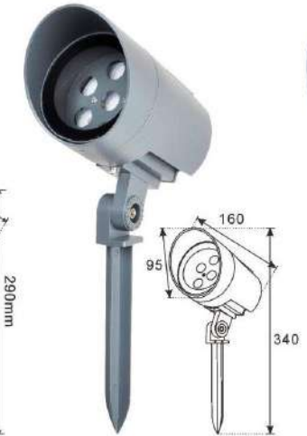
NO:YF-PZDC-10 18W 2900 Shell material: die cast aluminum Product size: 95x160xH340MM Aluminum substrate size: 75MM Power: 6x3W/9x2W Power box size: 70x38xH60MM
