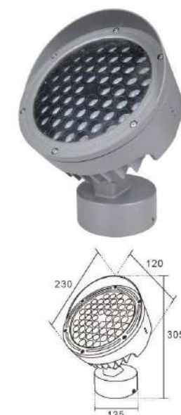
NO:YF-xHDZ-08 72W 7820 80W 8165 Shell material: die cast aluminum Product size: 230x120x305MM Aluminum substrate size: 190MM Power: 36x2W/54x1.5W Power box size: 135x70xH47MM
