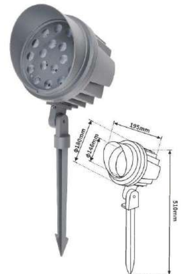
NO:YF-PZDC-15 30W 6325 Outer diameter size: Φ180MM Inner diameter: Φ146mm Power: 18W/24W Shell material: die cast aluminum
