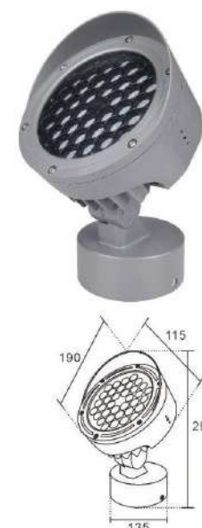
NO:YF-xHDZ-07 48W 5750 54W 6670 Shell material: die cast aluminum Product size: 190x115x290MM Aluminum substrate size: 150MM Power: 24x2W/36x1.5W Power box size: 135x70xH47MM
