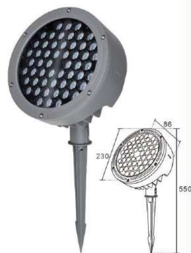
NO:YF-xHDC-04 72W 7705 80W 8050 Shell material: die cast aluminum Product size: 230x86x550MM Aluminum substrate size: 190MM Power: 36x2W/54x1.5W Power box size: 135x70xH47MM
