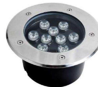
NO:YF-DMD-06 1680 1565 Outer diameter size: Φ180x90MM Inner diameter: Φ112MM Hole size: Φ158MM Power: 9W/12W Shell material: die cast aluminum
