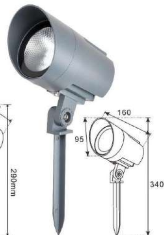
NO:YF-PZDC-06 20W 2760 Shell material: die cast aluminum Product size: 95x160xH340MM Aluminum substrate size: 75MM Power: COB 18W/20W Power box size: 70x38xH60MM
