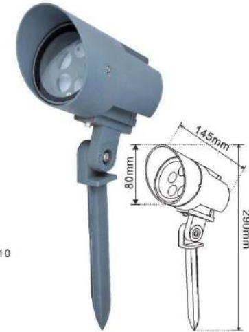
NO:YF-PZDC-09 3W 1795 5W 1890 10W 2070 Shell material: die cast aluminum Product size: 80x145xH290MM Aluminum substrate size: 62MM Power: 3W/5W/6Wx2 Power box size: 60x25xH50MM
