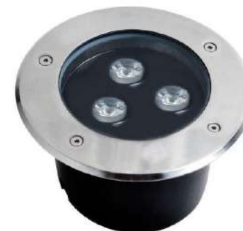
NO:YF-DMD-03 1035 Outer diameter size: Φ100x80MM Inner diameter: Φ62MM Hole size: Φ95MM Power: 3W Shell material: die cast aluminum
