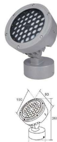
NO:YF-xHDZ-03 48W 5635 54W 6555 Shell material: die cast aluminum Product size: 190x80x260MM Aluminum substrate size: 150MM Power: 24x2W/36x1.5W Power box size: 135x70xH47MM
