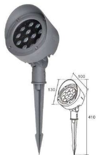
NO:YF-xHDC-05 18W 3220 24W 3565 Shell material: die cast aluminum Product size: 130x100x410MM Aluminum substrate size: 90MM Power: 9/12x2W Power box size: 90x40xH30MM
