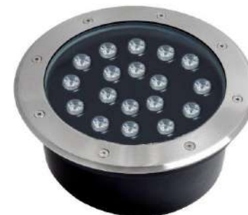
NO:YF-DMD-08 2415 2530 Outer diameter size: Φ220x90MM Inner diameter: Φ162MM Hole size: Φ208MM Power: 18W/24W Shell material: die cast aluminum
