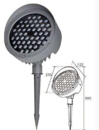
NO:YF-xHDC-08 72W 7820 80W 8165 Shell material: die cast aluminum Product size: 230x120x580MM Aluminum substrate size: 190MM Power: 36x2W/54x1.5W Power box size: 135x70xH47MM
