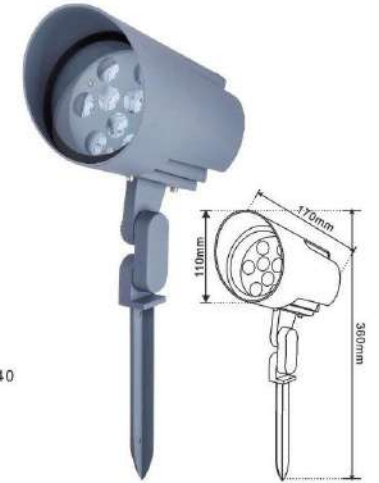
NO:YF-PZDC-11 18W 3130 24W 3565 Shell material: die cast aluminum Product size: 110x170xH360MM Aluminum substrate size: 90MM Power: 9W/12Wx2 Power box size: 78x46xH68MM
