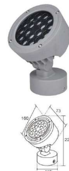
NO:YF-xHDZ-02 24W 3795 36W 4535 Shell material: die cast aluminum Product size: 160x73x225MM Aluminum substrate size: 120MM Power: 12/18x2W Power box size: 123x50xH40MM
