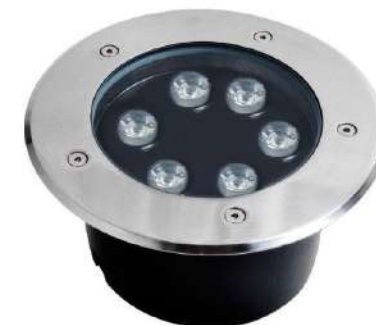
NO:YF-DMD-04 1220 Outer diameter size: Φ120x90MM Inner diameter: Φ83MM Hole size: Φ115MM Power: 6W Shell material: die cast aluminum
